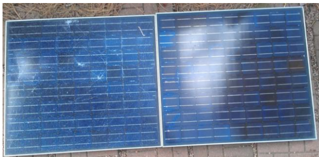
Photo 4: Side by side broken and good quality modules.
