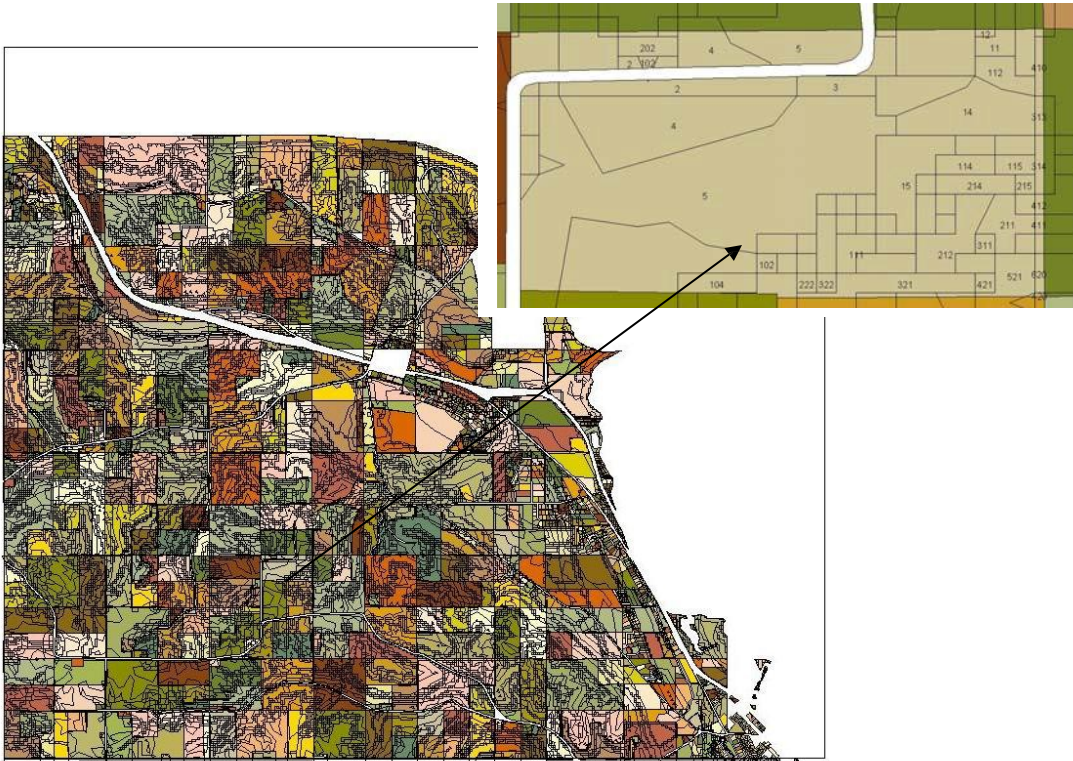
Figure 8. The composite shapefile was intersected with the parcels layer resulting in multiple values for each parcel. Detail shows the composite values for one parcel.
